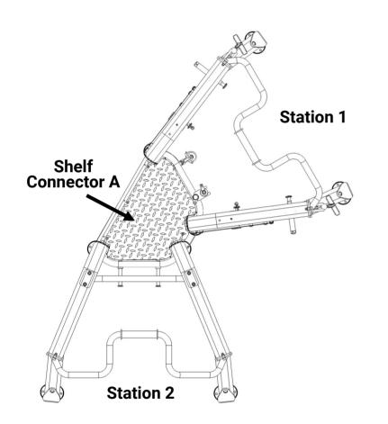
In order to prevent shifting or tipping: If installing and connecting any combination of two of the AXIS Free Trainer, The AXIS Bodyweight Trainer, AXIS Smith Trainer, or AXIS Freeweight Rack with the AXIS Shelf Connector A, both stations must be anchored to the floor using the AXIS FLOOR ANCHOR KIT before use.
